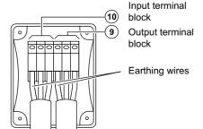
The overall cable diameter and the cross-sectional area of the three wires depends on the **UPS** rating.
